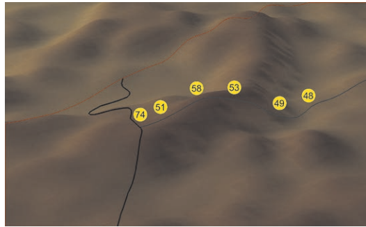
Figure 5. Values of average equivalent sound level ( L_{Aeq} ) in “Budzisko” profile at various distances from roadway edge Source: own study.
