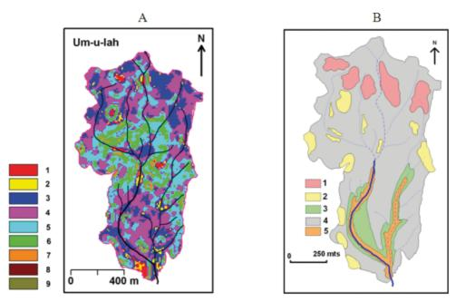
Figure 4. (A) Slope variations and (B) hydrological soil types in the experimental watershed
