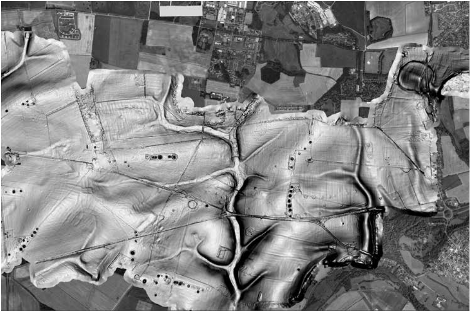
Fig. 1. DTM of the landscape of Stonehenge derived from terrestrial laser scanning
