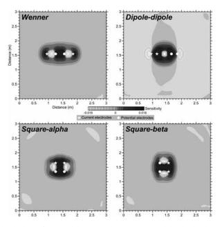
Fig. 1. Sensitivity depth slices of square-alpha, square-beta, Wenner and dipole–dipole arrays for a homogeneous earth model that has a resistivity value of 100 ohm-m. Depth is set to 0.25 m. Stars and circles indicate current and potential electrodes, respectively
