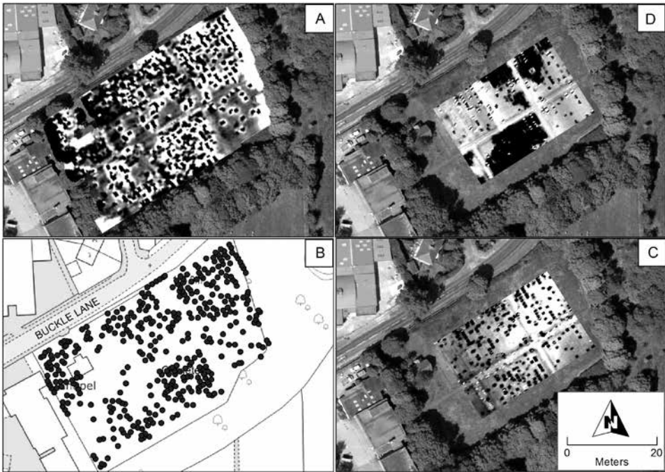
Fig. 2. Magnetic and electromagnetic results (plotted white [low] – black [high]). From top left: A – fluxgate gradiometer (-10 to 10 nT); B – fluxgate gradiometer anomaly centres of mass; C – electromagnetic conductivity, HCP C_i (-3 to 8 mS/m); D – electromagnetic in-phase HCP I_i (-0.5 to 1 ppt)
