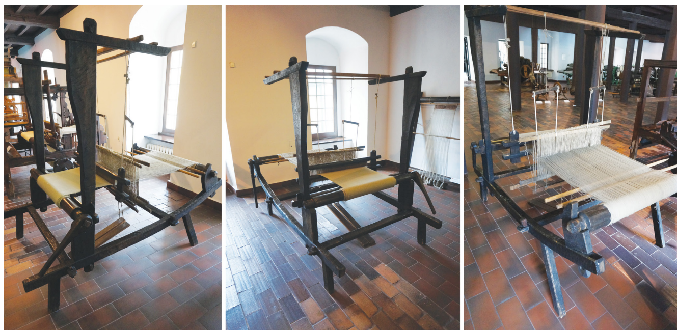
Fig. 6. Reconstruction of a horizontal treadle loom from Gdańsk by Adam Nahlik. On display in the Central Museum of Textiles in Łódź. Photo Ł. Antosik.
