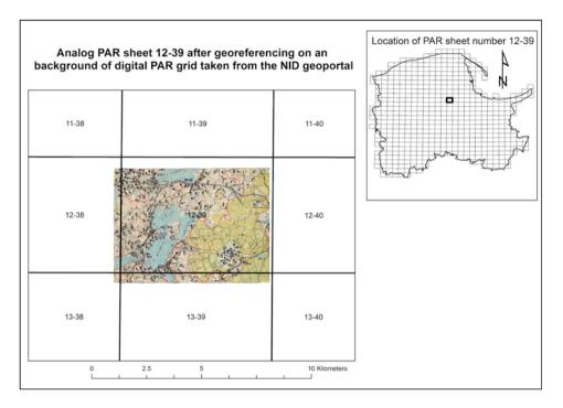
Fig. 5. Scan of analogue AZP sheet no. 12-39 georeferenced on a background of digital AZP grid taken from the NID geoportal
