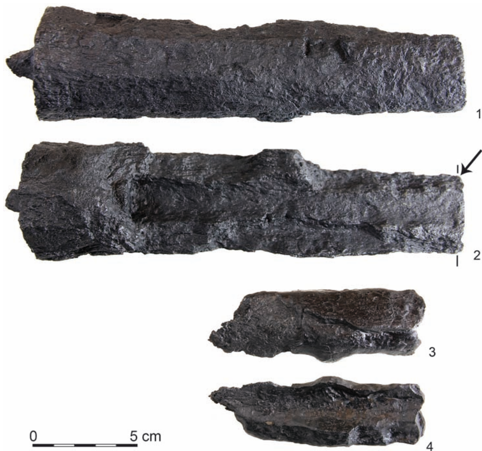
Fig. 4. Iron barrel fragments of the hackbut from Żelechów Castle: 1-2 – fragment of the breech section; 3-4 – fragment of the central section. Photo: W. Bis
