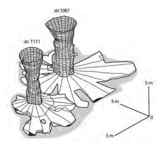
Fig. 3. Jablines 'Le Haut-Château', Seine-et-Marne district. 3D view of a deep flint mine. This pictorial allows not only to visualize the overlapping of the structures but also to determine the volume of bedrock that was removed and the quantity of raw material collected.
