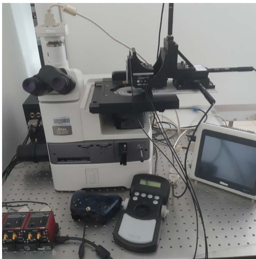
Figure 3.45: Microscope setup with microcontrollers used to deposit PCP onto the sample.
