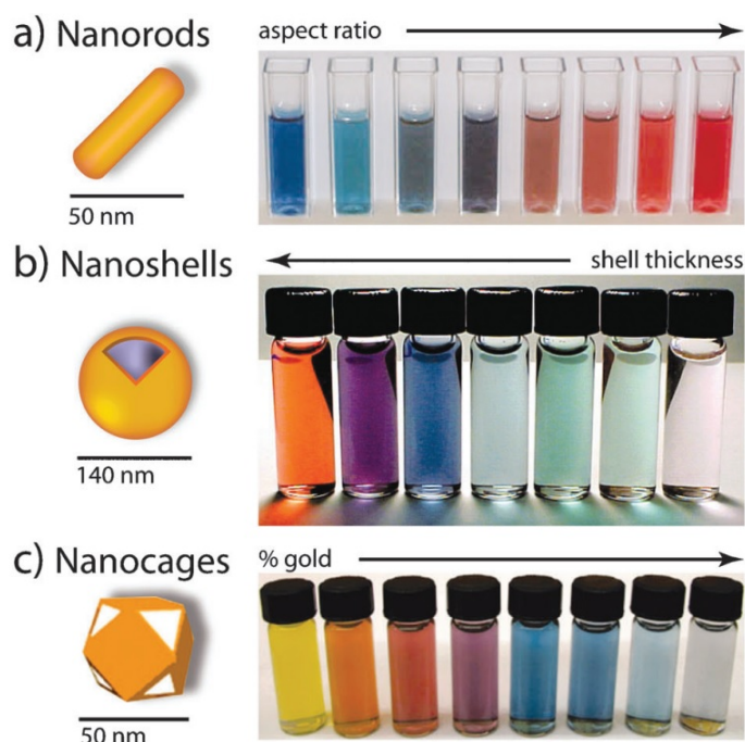
Figure 1.1: Photographs of AuNPs dispersions. In each solution AuNPs vary in morphologies, which results in variations in color of their dispersions[3].
