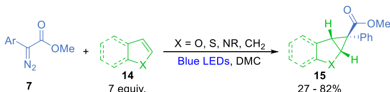
Scheme 8: Photochemical flow [2+1] cycloaddition of diazo compounds with carbo- and heterocycles.
