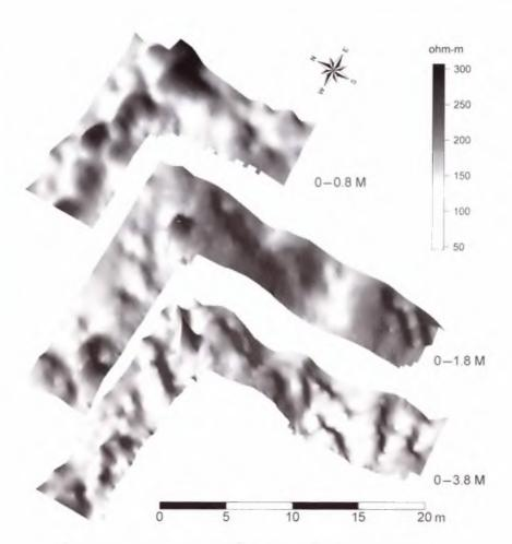
Fig. 7. Tanais. Research in 2002. Depth slices (3D) of the resistivity survey.
