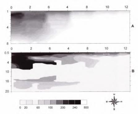
Fig. 10. Tanais. Research in 1997. A – apparent resistivity pseudo-section; B – geoelectrical cross-section.
