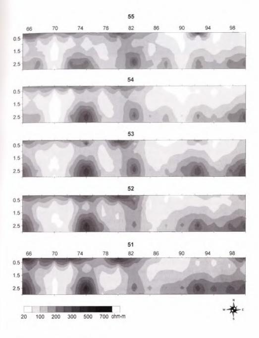
Fig. 4. Tanais. Research in 1998. Depth slices of the resistivity survey. Fig. 5. Tanais. Research in 1998. Apparent resistivity pseudo-sections.
