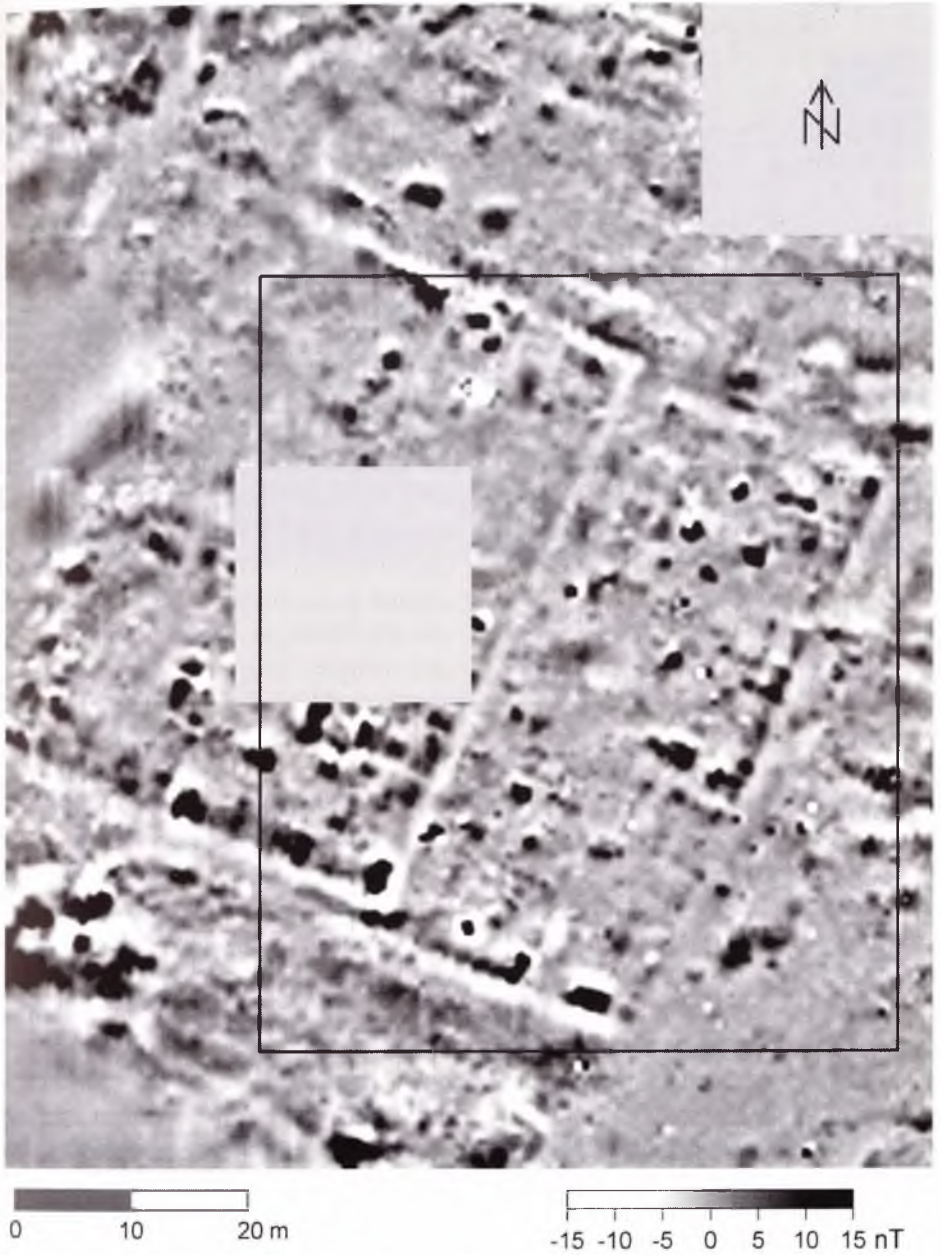
Fig. 26. Dakhleh Oasis, Ain el-Gazareen. Magnetic map of the western part of a large enclosure and the eastern enclosure (measurements by fluxgate gradiometer FM 36), sampling interval 0.5 by 0.5 interpolated to 0.25 by 0.25 m. The rectangular frame in the picture corresponds to the area covered in Fig. 27.
