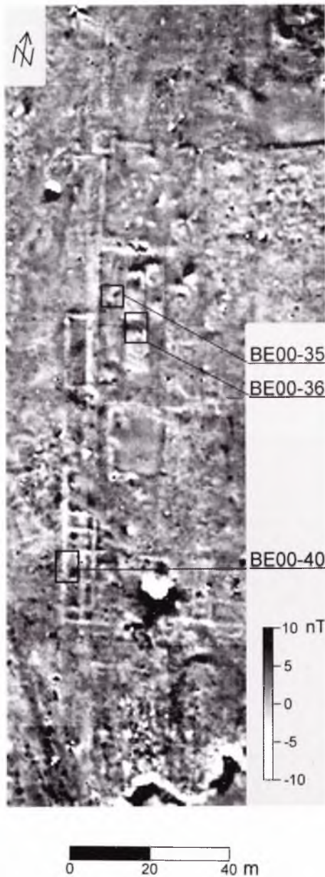
Fig. 30. Berenike. Magnetic map and location of test trenches. Sampling interval 0.50/0.50 m interpolated to 0.25/0.25 m.
