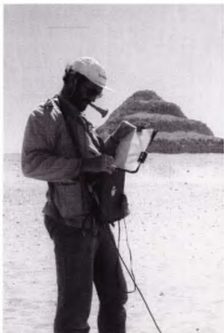
Fig. 3. Saqqara, west of the Djoser funerary complex. Measurements with a proton magnetometer PMP-4. A child's horn served to synchronize the traversing and stationary apparatus.
