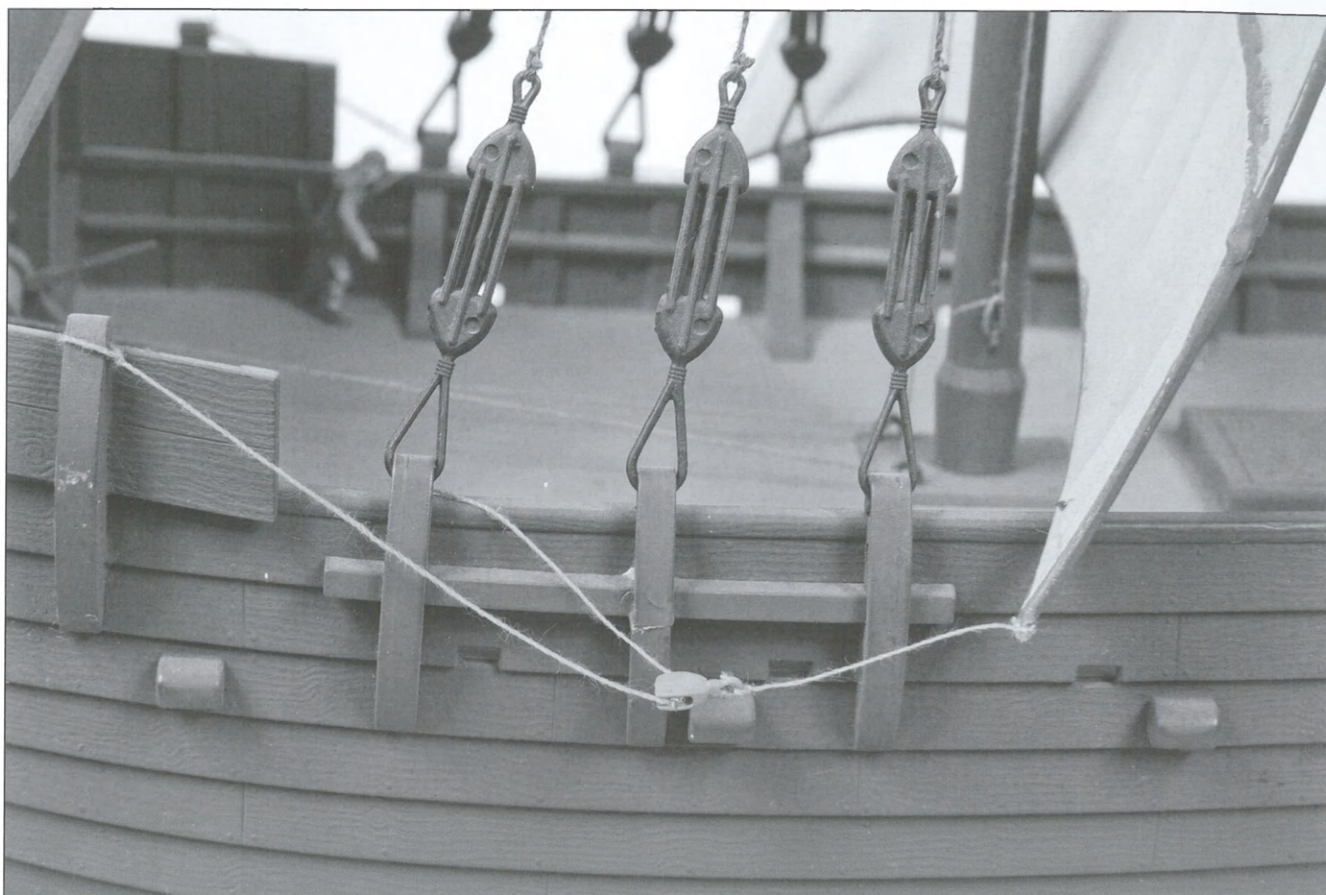
Fig. 6. Ways of fixing the shrouds (Photo by J. Słomska).
