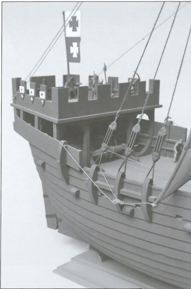
Fig. 7. Structure of the sterncastle, the windlass for raising the yards below (Photo by J. Słomska).
