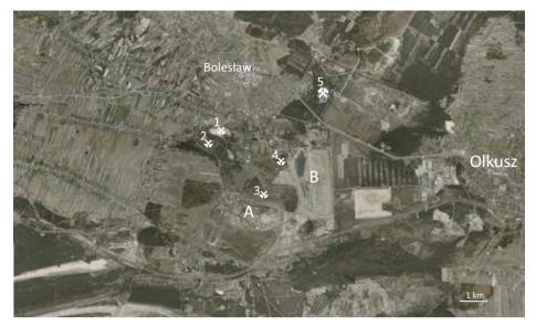
Fig. 6. A satellite picture of the mining area of the Bolesław Mining and Metallurgical Plant in 2019 with marked locations of reclaimed open-pit mines: 'Bolesław' (1), 'Krążek' (2), 'Hałda Michalska' (3), 'Ujków Stary' (4), 'Dąbrówka' and the underground mine 'Olkusz-Pomorzany' (5). A – ZGH Bolesław zinc smelter, B – ZGH Bolesław settling ponds [Orthophotomap originate from the National Geodetic and Cartographic Resources (PZGiK)]
