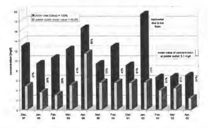
Figure 5. Measured suspended particulate matter concentrations at polder inlet (dark columns) and outlet (light columns).
