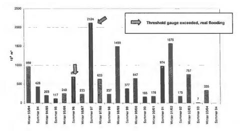
Figure 10. Water volume flowing through Polder A/B during the course of a decade. Winter flooding: November – April; (hypothetical/real) Summer flooding: April – November.
