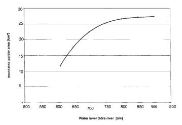
Figure 6. Correlation between flooded polder area and Odra gauge based on a digital elevation model
