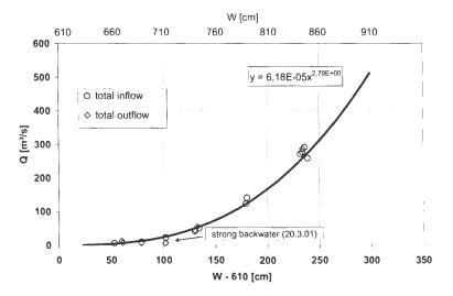
Figure 3. Correlation between measured polder discharge and Odra river water level at inlet gauging station
