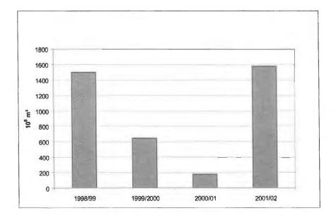
Figure 9. Water volume flowing through Polder A/B during winter flooding periods.
