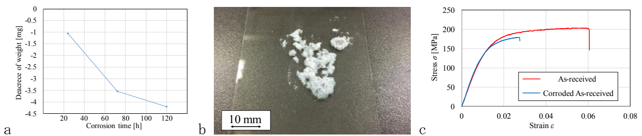
Figure 3: (a) The decrease of weight of As-received,(b) Corroded Mg/Ti, (c) The stress-strain curve of As-received.
