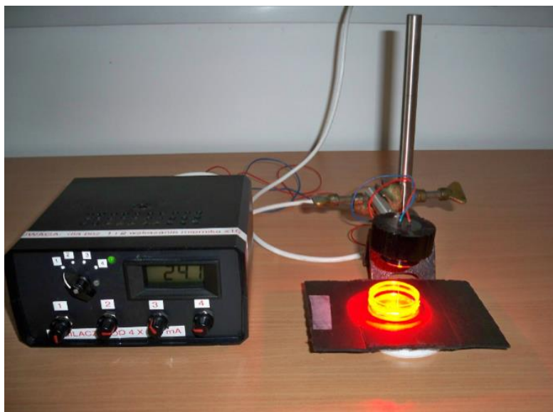
Figure 11. Home-built equipment for irradiation of the biological samples, with LED Array (Roithner Laser Technik, \lambda_{max} = 624 \text{ nm} , P = 120 \text{ mW} ).
